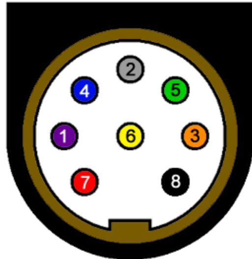
8-pin DIN Wiring Diagram (rear panel view)
